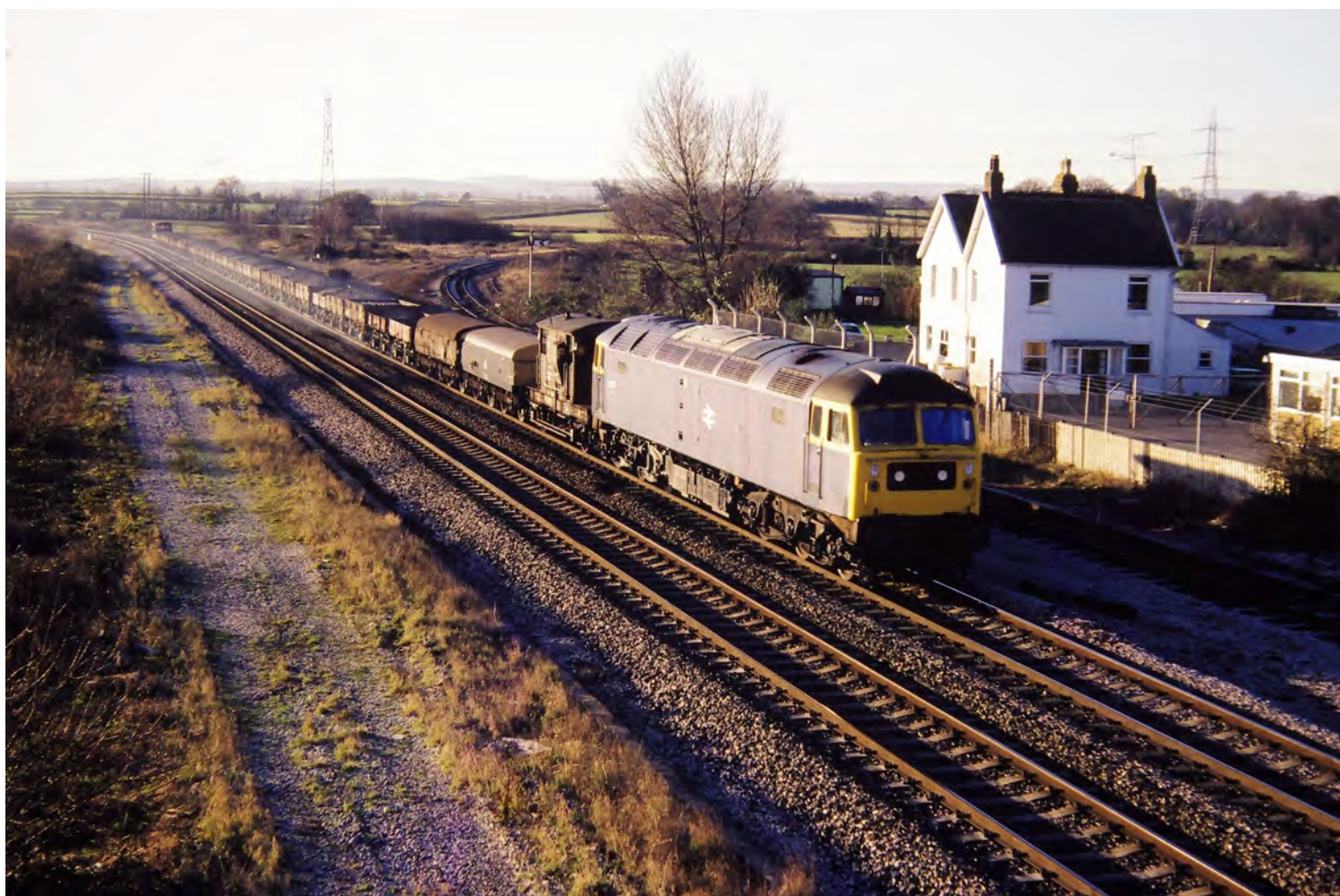
Photo: An up Ballast train headed by a class 47 locomotive passes the former Norton Fitzwarren station site in December 1980. The station hotel is to the right, and the actual derailment point is on the left, near the end of the ballast road which follows the route of the down relief line. Note the twin brake vans and two brake tenders in the consist, to help provide brake force for this heavy train, which probably is otherwise unfitted, with no continuous brakes on the ballast wagons themselves.
